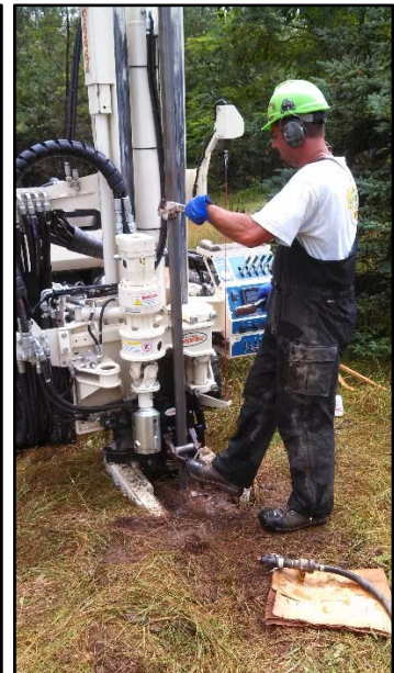
Photos 6 and 7: Subsurface borings will be collected using a Geoprobe drilling rig, allowing for physical measurement of depth-to-bedrock.
