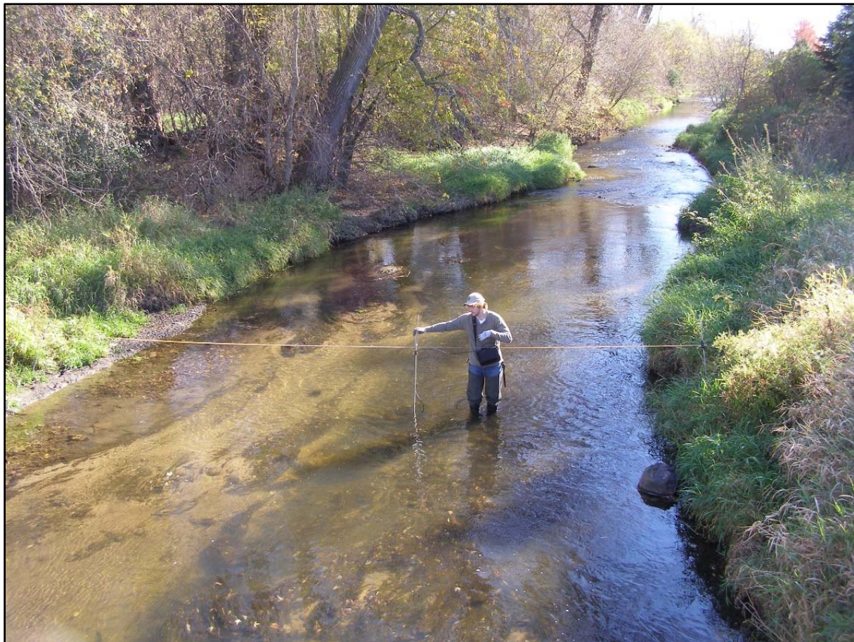
Photo 10: Streamflow measurements will be measured directly in stream channels using Acoustic Doppler Current Profiler (ADCP) equipment. In this photo, the field technician is collecting one of several measurements along a stream transect.
