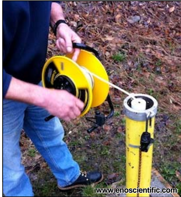
Photos 8 and 9: Water-levels in wells will be measured using a sonic water-level meter (photo to left) or a submersible water-level meter (photo to right).
