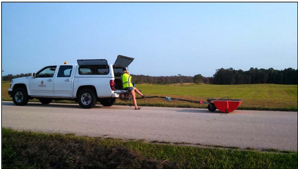
Photos 3 and 4: The 80 MHz Ground Penetrating Radar (GPR) equipment during set-up (above) and in action on the roads in the Town of Lincoln (below). This unit is typically pulled behind a pickup truck along roads or open fields at slow speeds (about 5 mph).
