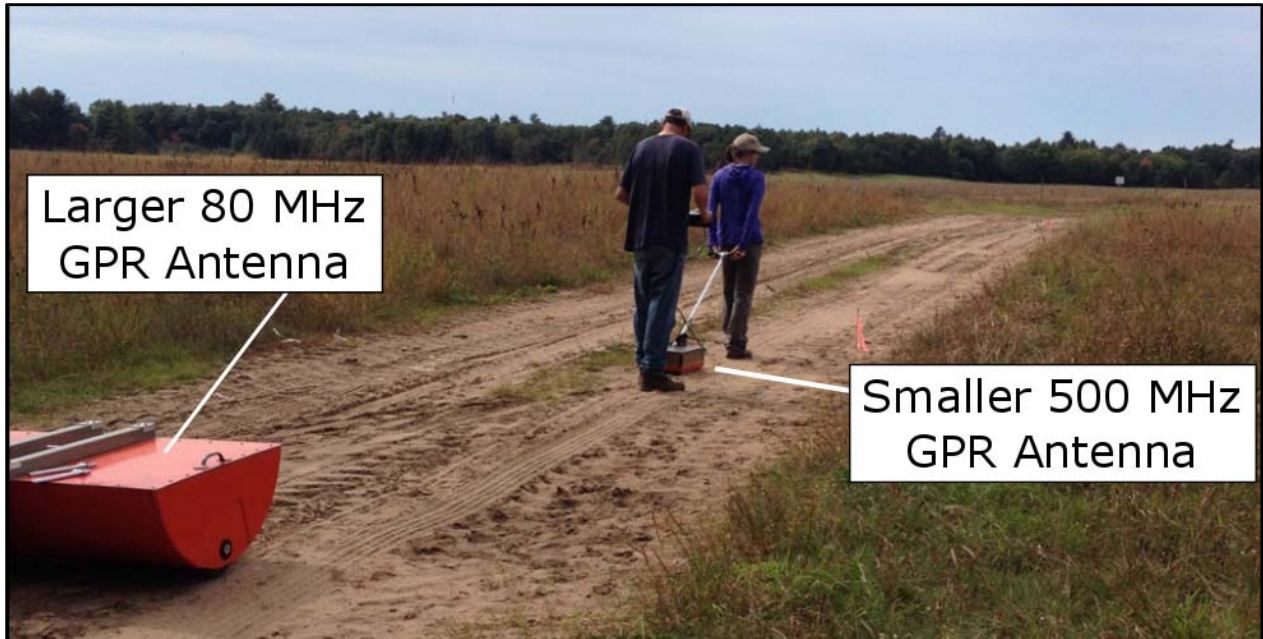
Photo 5: The smaller 500 MHz Ground Penetrating Radar (GPR) antenna can be used wherever the larger 80 MHz antenna can be used; however, it is smaller and can easily maneuverable in tight areas, such as in a field between rows of corn. The 80 MHz might temporarily flatten taller standing grasses and weeds, but they usually recover after a day. If the 80 MHz is being towed by truck, the minimal damage would be a result of the truck.
