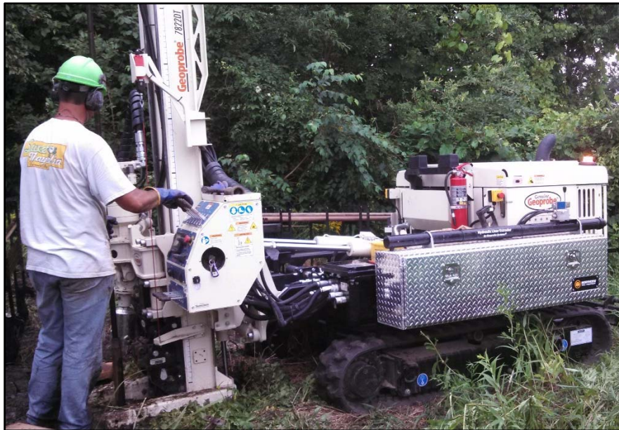
Photos 6 and 7: Subsurface borings will be collected using a Geoprobe drilling rig, allowing for physical measurement of depth-to-bedrock.
